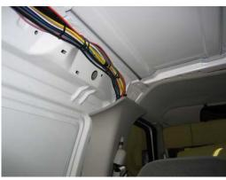
Run all wiring for dome lights, power vents, video system, HVAC, etc. at this time. Tie to existing OEM harness
